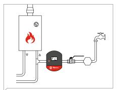
Flexcon PA with app and permanent connection to water pipe. The service technician installs the device along with an extra water hose, ball valve and backflow protection. To refill, the customer only has to open the valve.
