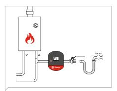
Flexcon PA with app. The service technician connects the device to the central heating unit. When necessary, the customer refills the system by connecting a hose to the central heating system.
