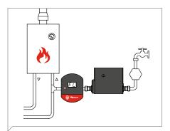
Flexcon PA AutoFill with app. The technician installs a fully-automatic unit. Refilling occurs automatically. AutoFill receives a signal whenever the Flexcon PA deems it necessary to refill the system. The customer does not have to do anything.
