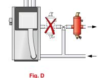
Place the product upstream of the boiler in the return line, if dirt separation is the primary function (A, C). If the primary function is air separation (A, C) or a
