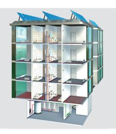
LogoComfort 600 Complete Units 50 are systems with proportional volume-controlled heat interface units that can be easily and quickly tailored to the requirements of your specific application.
