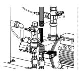
• Connect the supply line to the refilling supply. If necessary, install a dirt trap at the drinking water joint (0.2 mm).
