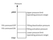
pMIN and pMAX are set on the working pressure limits and are not adjustable by the operator. pON and pOFF are adjustable within these limits.
