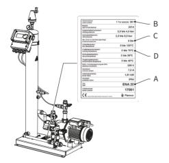
On the type plate the following product information can be found: A: Automat type (ENA 10, 20 or 30) B: Automat serial number C: Permissible working overpressure D:Permissible working temperature
