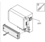
Switch off the power switch on the controller SCU.
