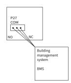
If controller powered down, than the is P27 normally open If controller is powered up, than the is P27 normally closed If controller is in error, than the is P27 normally open
