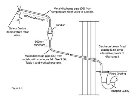
Note: It is not acceptable to discharge straight into a soil pipe.
