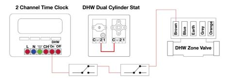
The link must be installed between the adjustable thermostat and the safety cut-out thermostat as shown above. The working thermostat which controls the temperature of the domestic hot water is adjustable. A safety cut out is also incorporated within the thermostat and will operate at  $85^{\circ}C \pm 3^{\circ}C$ . Both thermostats should run in series. To reset the safety cut-out and the motorised valve the reset button must be pressed in.
