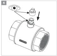
Plug the DIN adapter on the spindle. The marking on the shaft adapter must be parallel to the flank on the spindle.
