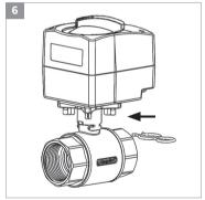
Attach the spring clip to secure the adapter.
