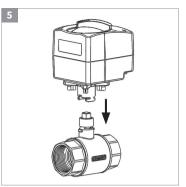
Plug the actuator on the ball valve.
