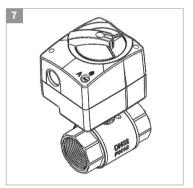
Position display: **Red:** Ball valve is opened, **Blue:** Ball valve is closed Initially adjust the switch from Auto to Manual for manual actuation.
