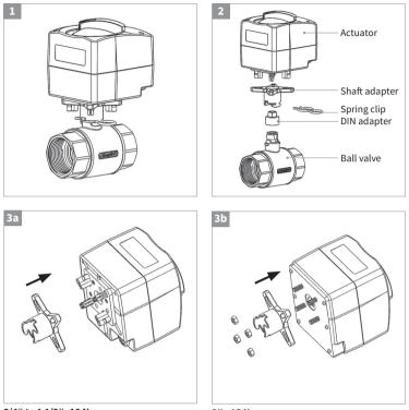
**3/4" to 1 1/2"- 10 Nm:** Plug the shaft adapter drive on the actuator
