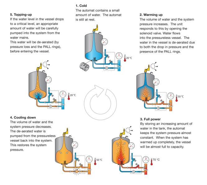
The vessel is tested to 2 bar, however in operation it is an atmospheric vessel, essentially a water balloon in a protective shell. The water within the vessel has no pressure other than its own vertical weight.
